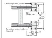
The dimensions of the fixed point and driver connections are identical.
